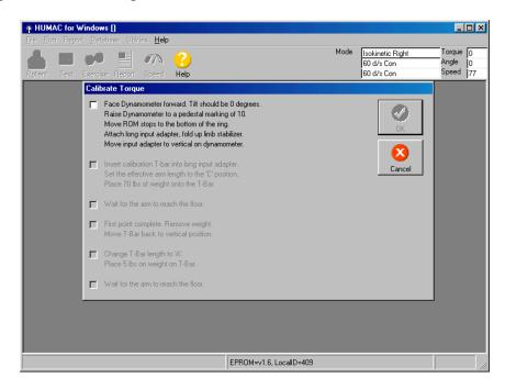
2. Insert the calibration bar into the adapter at the <u>C setting</u> and place 70 pounds to the bar. When you check this box, the HUMAC will set the CYBEX speed to 12 deg/sec and the weight will begin to fall. Place about 20 lbs of resistance on the bar to prevent bouncing through the first third of descent.
