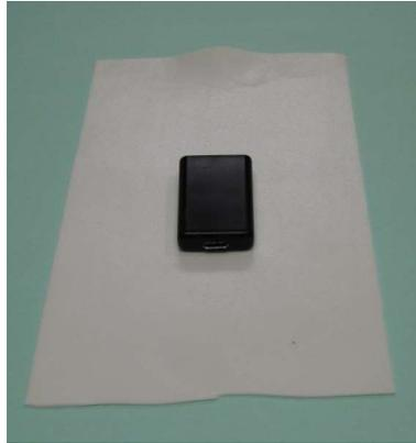
Appendix 5, Figure 2a. AX3 face down on adhesive side of 5” by 4” of tape
