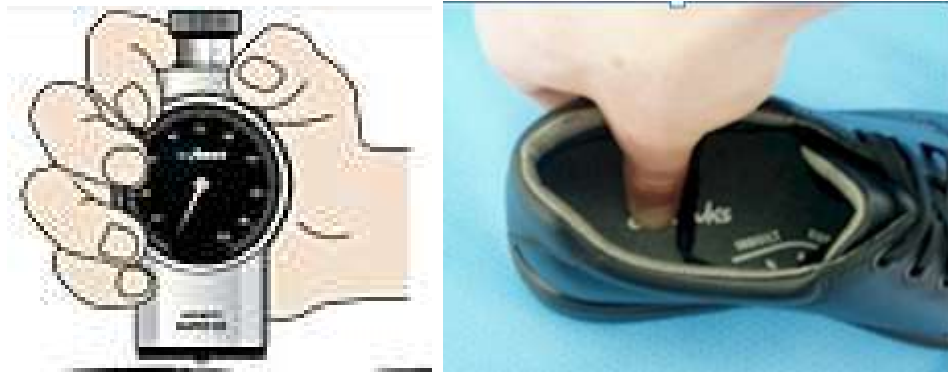
Figure 2. Shoe hardness assessment using Shore A durometer. Hold the Shore A durometer as shown (left). With the indenter at the lateral heel-shoe interface as shown on the right, press on the indenter until all slack has been taken up. Record the reading from the position of the red needle.
