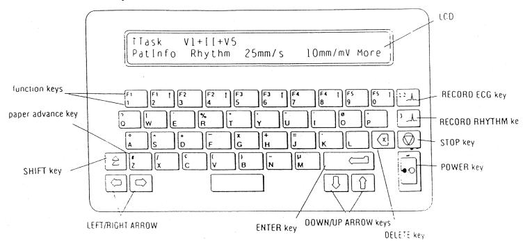
Note: Each of the 10 numerical keys on the keyboard has a number from 1-5 on it preceded by the letter F. These keys are dual purpose: They are used to either type in numerical data or as a function key to select an item from the LCD.
