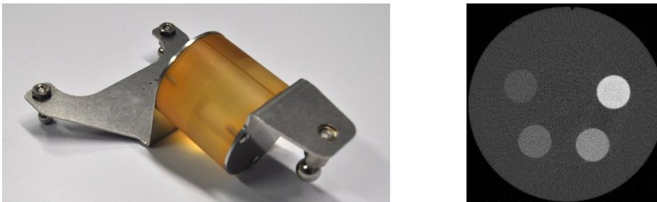
**Figure 3-2:** Scanco XtremeCT II QC phantom
